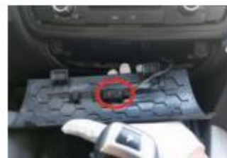
6. Unplug the lower cover light of the host.
