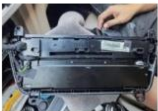
9. Install the Radio panel and fix the aftermarket Panel in place.
