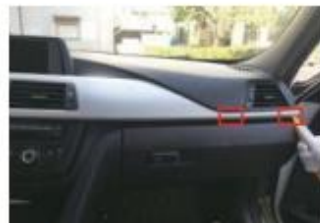
2. Pry loose the decorative sheet of air-conditioning.
