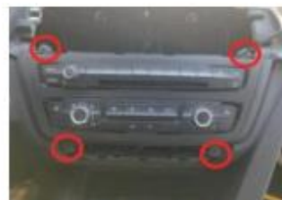
7. Take out the fixing screws of the host panel (with T20 screwdriver).
