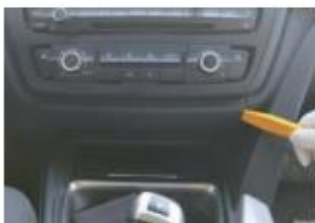
5. Pry and take out the lower cover of the HOST.
