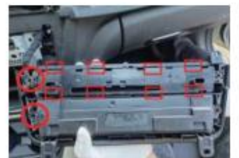
8. Unplug the Radio and Air conditioner panel, then pry loose the buckle from 8 positions and take out the original car radio panel.
